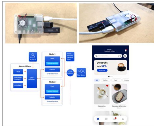
Figure 3. Prototype and System Topology of Pocket Data Centre
